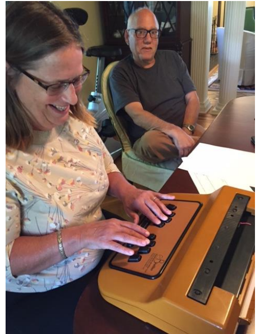
Lead teacher Barbara Games using COSMO as a stand-alone Braille writer/embosser. Dave Pillischer instructs.
